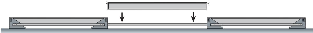
Figure 2-2. Spacer Tube Installation
