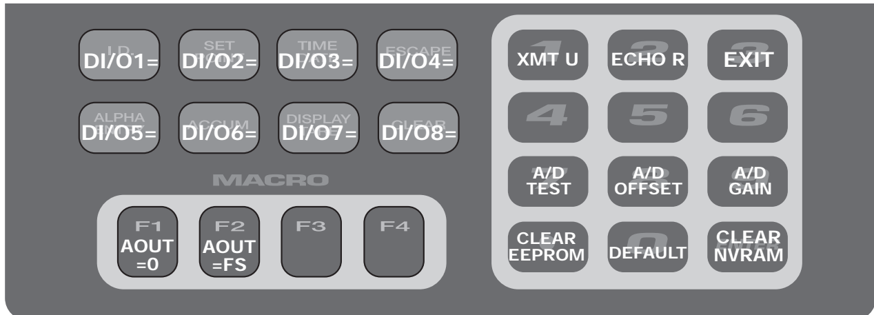
Figure 10-6. Front Panel Key Functions in Test Mode
